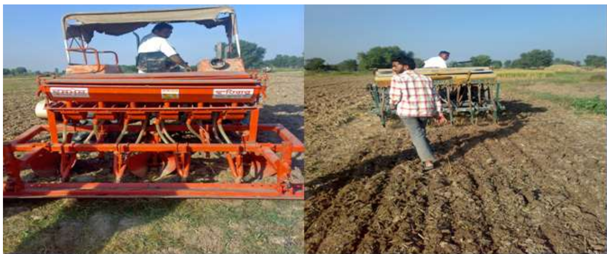
Resource conservation technologies through Bed planter and Zero till Seed drill
