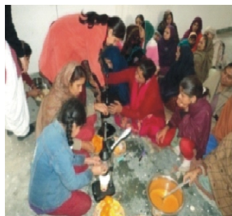
Processing of Kinnow into squash (Extraction of juice, Filtering, Filling of squash)
